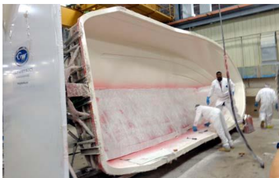
Adding fiberglass to the gelcoat
