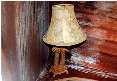
A closed boat in a warm and muggy area can lead to this. (Photo: BoatUS.)
