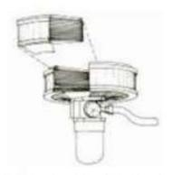
Just like a car engine, a boat engine can backfire. Any boat that is fueled by gasoline needs to have a backfire flame arrestor equipped for this reason. With the exception of outboard motors, that is. The backfire flame arrestor needs to be installed on a carburetor to function.
