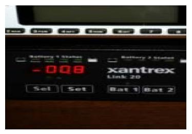
Note GWTW is equipped with a main battery bank composed of 4 6volt golf cart batteries hooked up in a series/parallel fashion to give her 440 amp hours. The link monitor is set to ½ that at 220 amp hours so there is plenty of reserve power. She is also setup with a 120 amp alternator and a regulator with a combiner to keep the batteries charged when running the iron jenny.
