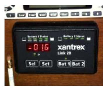
The following picture shows my system at rest. Here you will note with nothing at all on the boat that it shows a 0.1 amp draw that is the Xantrex link monitor. This draw is on all the time whether the main switch is on or off. I've made a note to offset that draw with a solar panel in the near future as that equals a 02.4 amp hour draw in 24 hours or 16.8 amp hours within a 7 day period.
