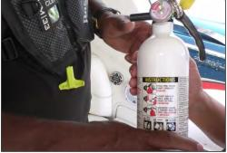
Disposable dry chemical extinguishers expire 12 years after their date of manufacture, and rechargeable extinguishers expire annually unless maintained by a certified technician.
